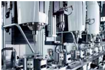
Fig 1: Sequence of honing and measuring station in a multi-spindle transfer honing machine. The interior of a highly productive honing machine in transfer design. Each honing station is followed by a measuring station. With the captured processing results, it is possible to keep the honing quality within an ideal range via a control loop.
