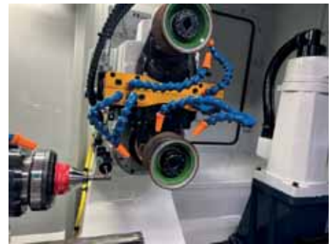
Measurement of the tool for runout compensation by means of a measuring probe
