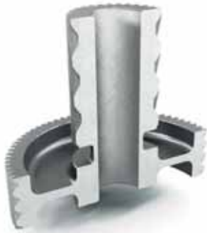
Fig. 3: Application example 1 - Planetary gear for electric vehicle transmission with through hole to be honed. Components like this one very often show different elastic deformation during machining due to uneven material distribution.
