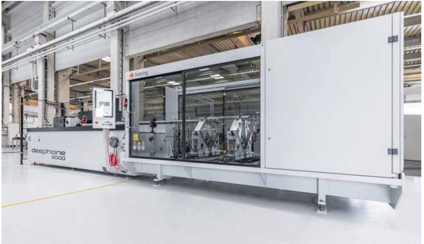
Gehring supplies deephone machines for large precision tube components with stroke lengths of 2-10 m. Internal and external machining is possible. The Gehring operator panel supports the operator with intuitive menu guidance.
